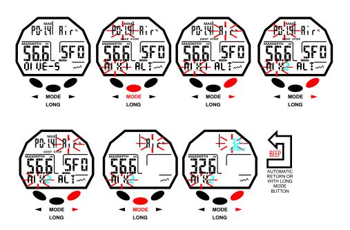
type of mixture contained in the cylinder and to set the FO2 of the computer according to that mixture.
