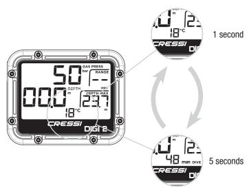
When the dive is complete, two minutes after reaching the surface (depth < 0.8 m), the DIGI 2 console switches back to surface mode (see chapter SURFACE SCREEN [PRE-DIVE]). Thus it will show the following information:
