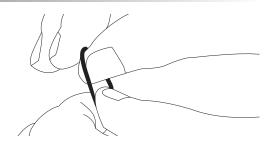
3. Change the O-ring on the closure cap with a new one, and grease it lightly, using silicone grease ONLY.
