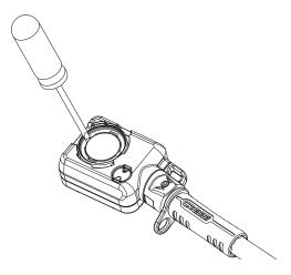
4. Gently insert a pointed object (a small flat-head screwdriver) into the cavity, and carefully and delicately lever up the used battery.
