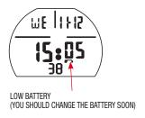
If the flashing battery icon appears on the display, the dive functions will be disabled for safety reasons.
