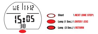
**Short:** when pressed briefly, the button scrolls through the various menus and sets the adjustments in increments. When pressed **Long** (1 second) the button enters the various menus and confirms; pressing even **Longer** (3 seconds) returns you to the previous menu.
